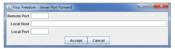
It is not absolutely necessary to use the same numbers for "remote port" and "local port", but we have found that many applications are too silly to announce another port to "the network" than they actually listen on. For example, BitTorrent clients usually can announce different external IP addresses and ports, but 99 % of all trackers will simply ignore this. So use the same port on both ends (by configuring your application accordingly) and it will all work by sheer magic.
